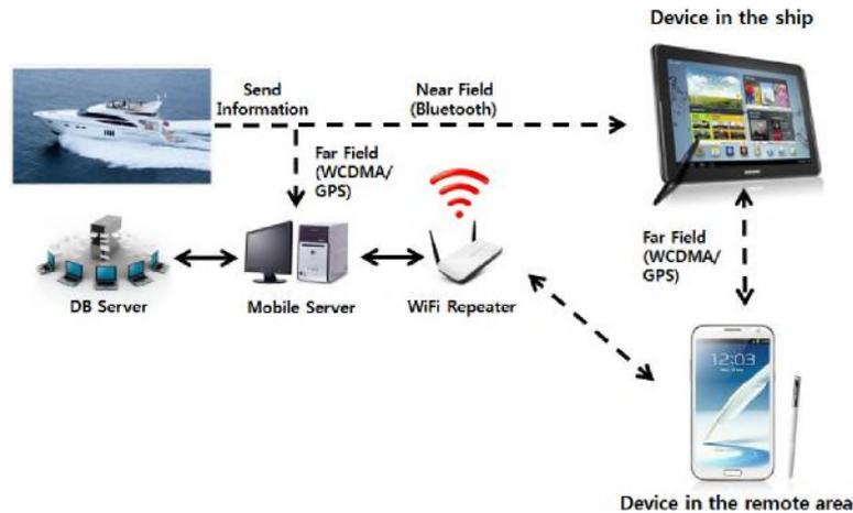
**Fig. 1.** Concept of the smart vessel platform
