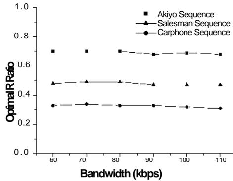
Fig. 1. Optimal R Ratio comparison versus network bandwidth for Akiyo, Carphone, and Salesman sequences.
