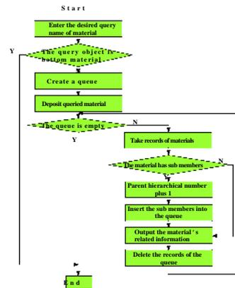
Fig. 3. Flow chart of improved algorithm
