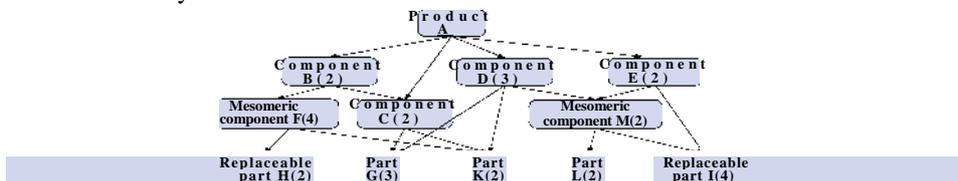
Fig. 1. The structure of cross-style BOM
