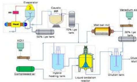
**Fig. 1.** The model of evaporation and liquid phase oxidation units using METSIM
