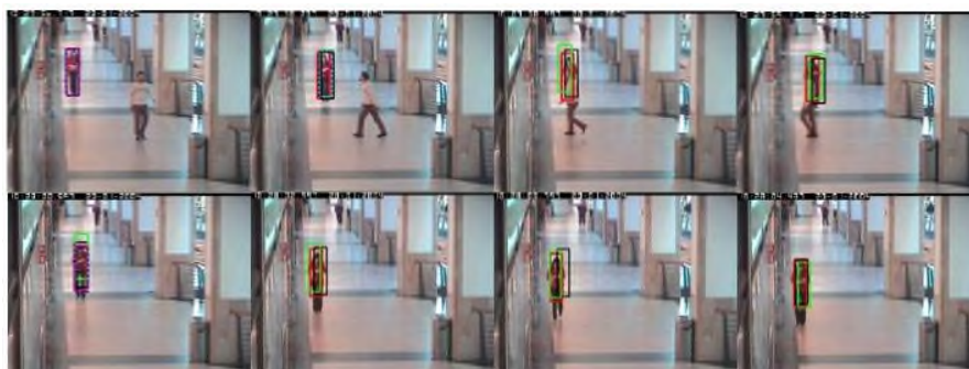
Figure11. Tracking Results of OneLeaveShopReenter1cor: Our tracker (red), MIL (green), Adaboost (black), Semiboost (dotted blue)
