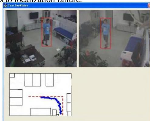
**Figure 14. Localization results using distributed vision system in [20].**
