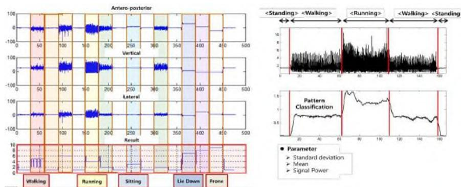
Fig. 3. Posture judgment algorithm by 3-axis acceleration sensor.
