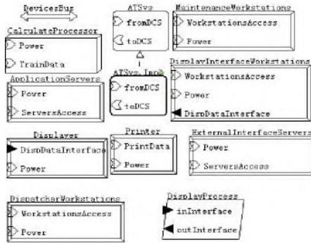
**Fig. 3.** the components in the ATS subsystem
