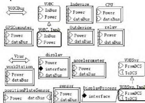
**Fig. 6.** components used in the vehicle on-board subsystem
