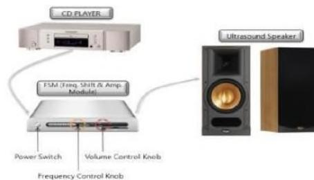
**Figure 4. Overall USS (Ultrasonic Speaker System) configuration**
