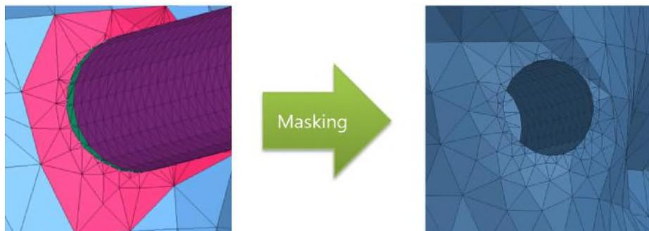
**Fig. 7.** Masking the Surface Mesh of Spine Model Copying Implant
