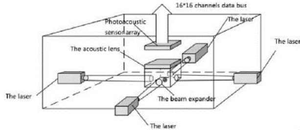
**Figure 10. Experimental System of Acoustic Lens Opto-acoustic Tomography**
