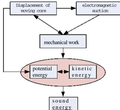
Fig. 6. the conversion relationship between work and energy during transition phase
