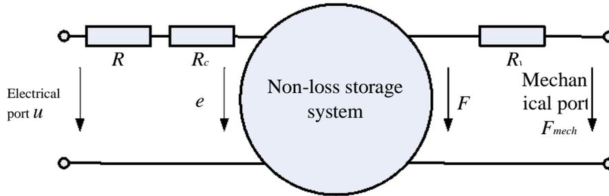
Fig. 2. Schematic of mechanical energy and electromagnetic energy conversion process
