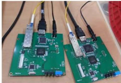
**Fig. 2.** HDMI - Fiber-Optic Interface board
