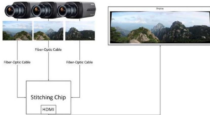
**Fig. 3.** Example of image stitching system
