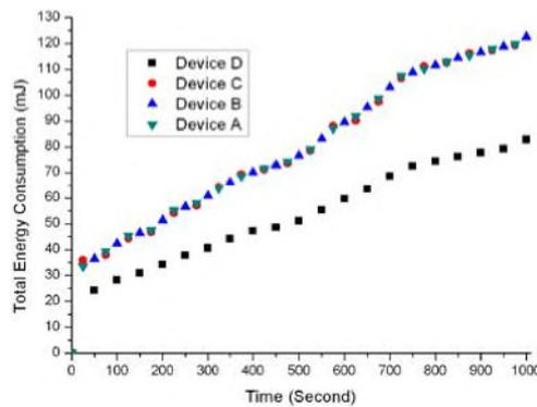
**Fig. 3.** Energy consumption of device according to the operating time of WiMedia device
