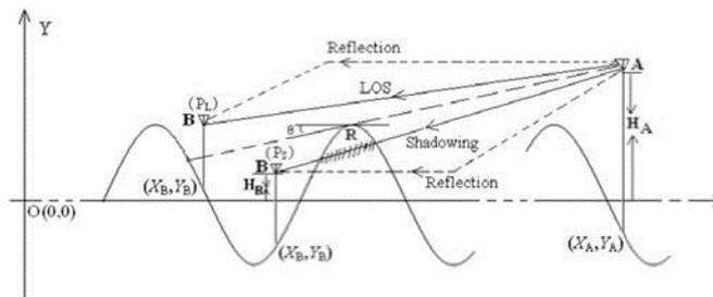
**Fig. 1.** Three types of signal propagation manners, i.e., LOS, shadowing and reflection propagation[3].
