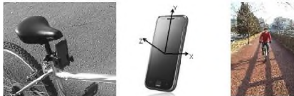
Fig. 1. Acceleration measurement using smartphone mounted at the same position as the embedded wrist-watch. (a) Mounted on a seat post (left), (b) Accelerometer axes (center) and (c) Riding experiments on a slope with 10^\circ inclination angle (right).
