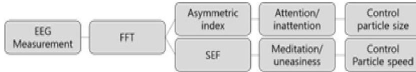
Fig.1. Process of BCI real-time fluid system
