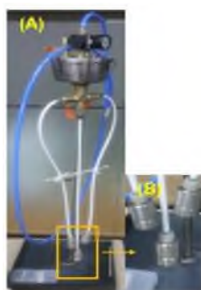
Fig. 3. Pictures of preparing equipment; (a) manufacturing equipment, (b) magnified corporate needles (diameter: 0.5mm)
