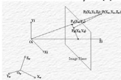
Fig. 3. Tasi camera calibration algorithm Camera calibration
