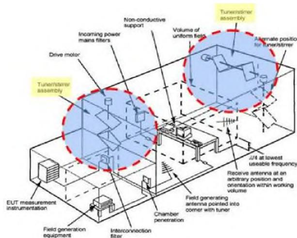
Fig. 1. Reverberation chamber and stirrer.
