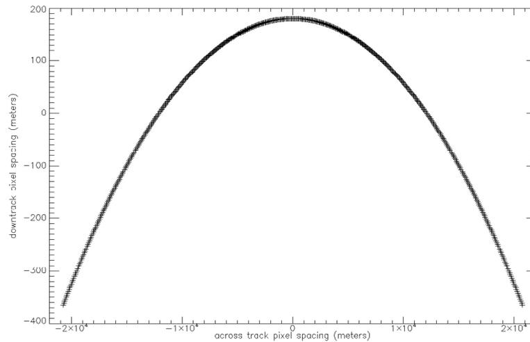
**Figure 1.** Preflight characterization of the curved slit projection in object space, showing the nominal pixel-center spacings after projection onto a horizontal surface from an elevation of 100 km.
