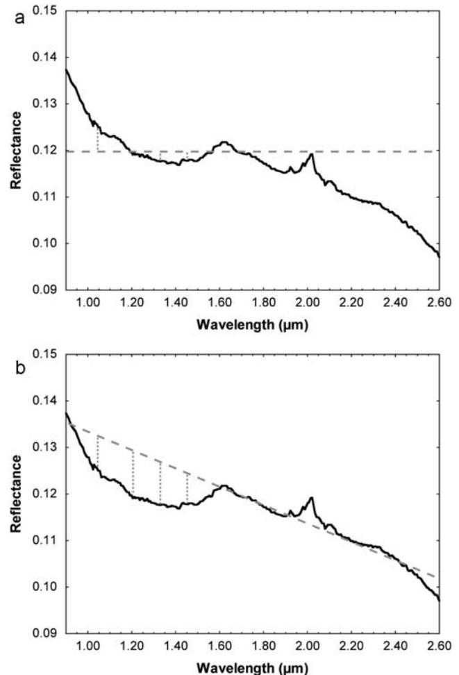
**Figure 2.** Comparison of the (a) original OLINDEX and (b) OLINDEX2. Olivine is only correctly identified when the slope of the spectrum is accurately modeled. The spectral peak near 2.00  $\mu\text{m}$  is an anomaly created by imperfections in the atmospheric correction.
