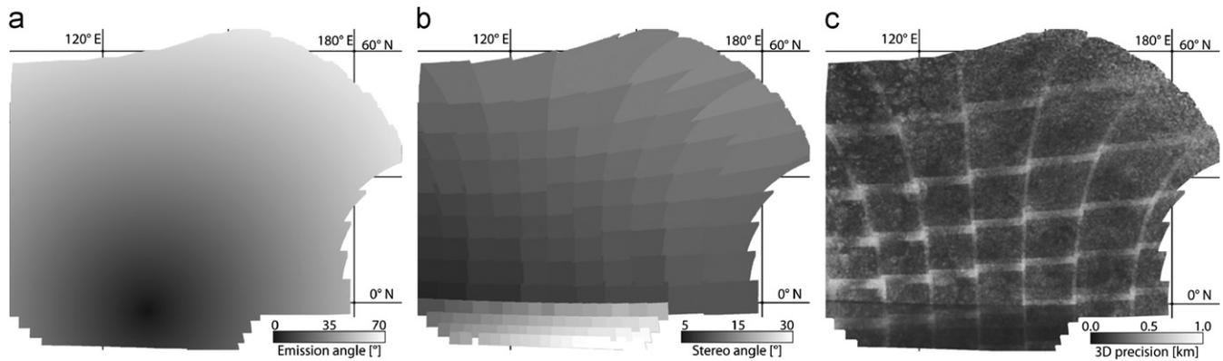
**Fig. 2.** (a) Graphical depiction of emission angles for images in the M1 departure mosaic, which was used to compute the M1 DTM. (b) Stereo convergence angles between the M1 departure mosaic and the two mosaics M1 H1 and M1 H2, all of which were used to compute the M1 DTM. (c) Three-dimensional (3D) point accuracies for the M1 DTM. The largest point errors (approximately 500 m) are well below the DTM grid size.
