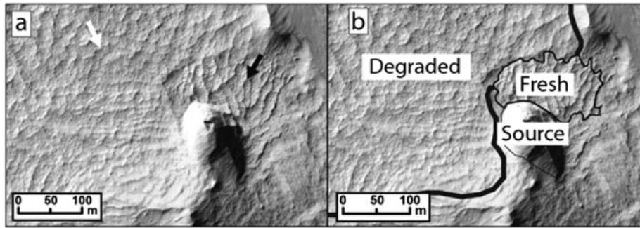
**Figure 11.** The transition from recognizable aeolian bedforms to degraded terrain. (a) A patch of fresh aeolian material (black arrow), interpreted to be eroding from the knob at center right, is superposed on older, indurated bedforms with subdued crests (white arrow) (Portion of HiRISE image PSP\_009398\_1685). (b) A sketch map outlining the units discussed in (a).
