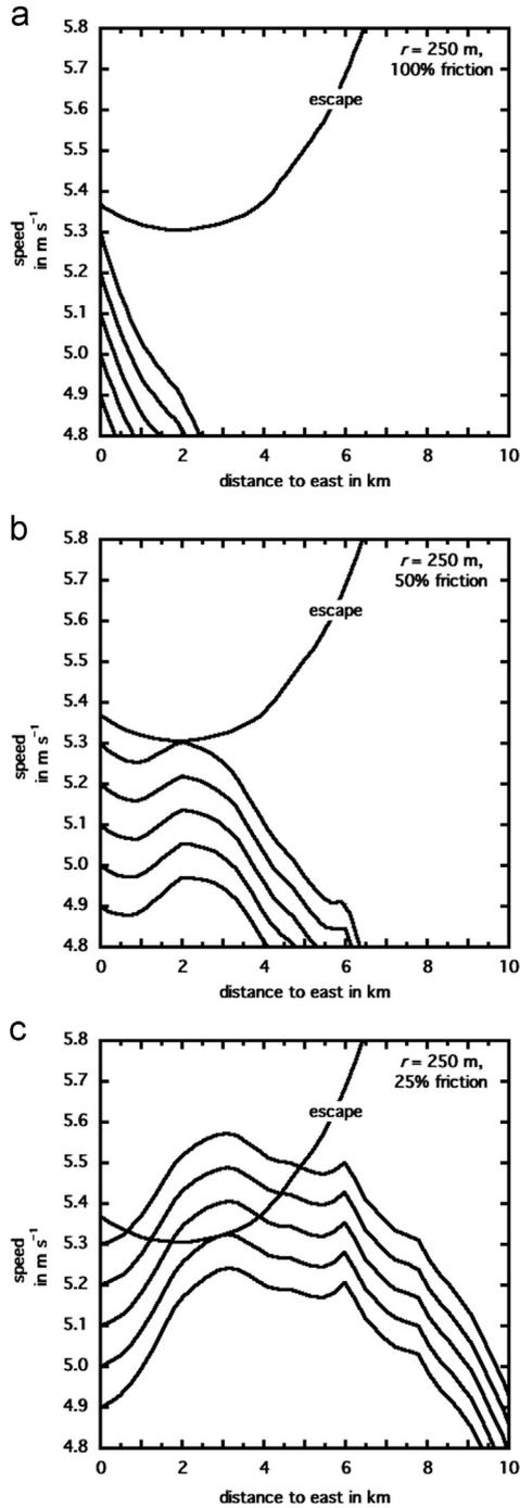
**Fig. 10.** Variation of boulder speed with eastward distance traveled from the vicinity of Stickney for a 250 m-radius boulder when the regolith friction is (a) 100%, (b) 50%, and (c) 25%, of the amount implied by Eq. (5). Initial boulder speeds are defined by the intersections of the curves with the speed ( $y$ ) axis.
