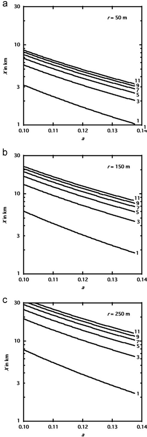
**Fig. 5.** The variation of boulder travel distance,  $X$ , as a function of  $a$  (boulder track depth–width aspect ratio) and initial speed,  $u_i$  (curves labeled 1, 3, 5, 7, 9, and 11  $\text{m s}^{-1}$ ), for clast radii of (a) 50 m, (b) 150 m, and (c) 250 m, calculated from Eq. (8) using a regolith density of  $1000 \text{ kg m}^{-3}$  and a clast density of  $1800 \text{ kg m}^{-3}$ .
