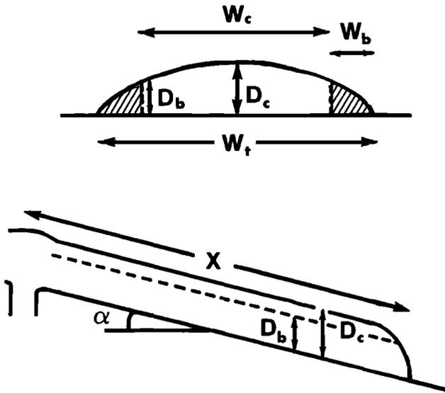
Fig. 6. The geometrical shapes of lava flows having the properties of Bingham plastics [Hulme, 1974]. The stationary banks on either side of the flow are shown shaded in the cross-sectional view perpendicular to the downslope flow direction. See text for definitions of parameters marked.
