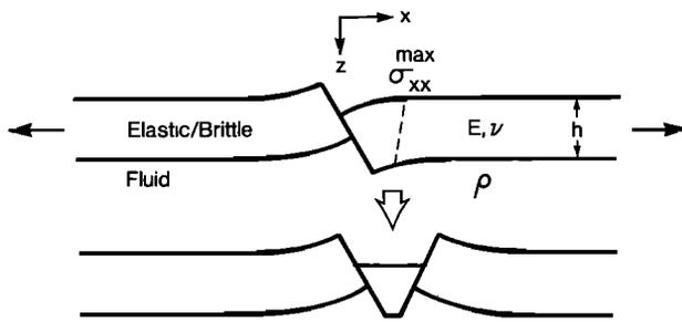
Fig. 6. The *Vening Meinesz* [1950] model for graben formation. Once a throughgoing normal fault forms in an extended elastic-brittle layer, then slip on that fault leads to additional bending stress in the layer. Under further extension, the preferred site for formation of the next failure plane will be where the surface bending stress  $\sigma_{xx}$  has its maximum extensional magnitude.
