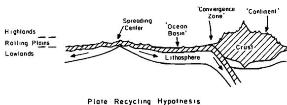
Fig. 2. A schematic illustration of the plate recycling hypothesis for lithospheric heat transport on Venus. The rolling plains (0 to 2 km elevation with respect to the planetary modal radius) and lowlands (0 to -2 km) are analogous to terrestrial ocean basins and include spreading centers and convergence zones not currently resolvable from altimetry or imaging data. The highlands (2 to 11 km elevation) are analogous to terrestrial continents.
