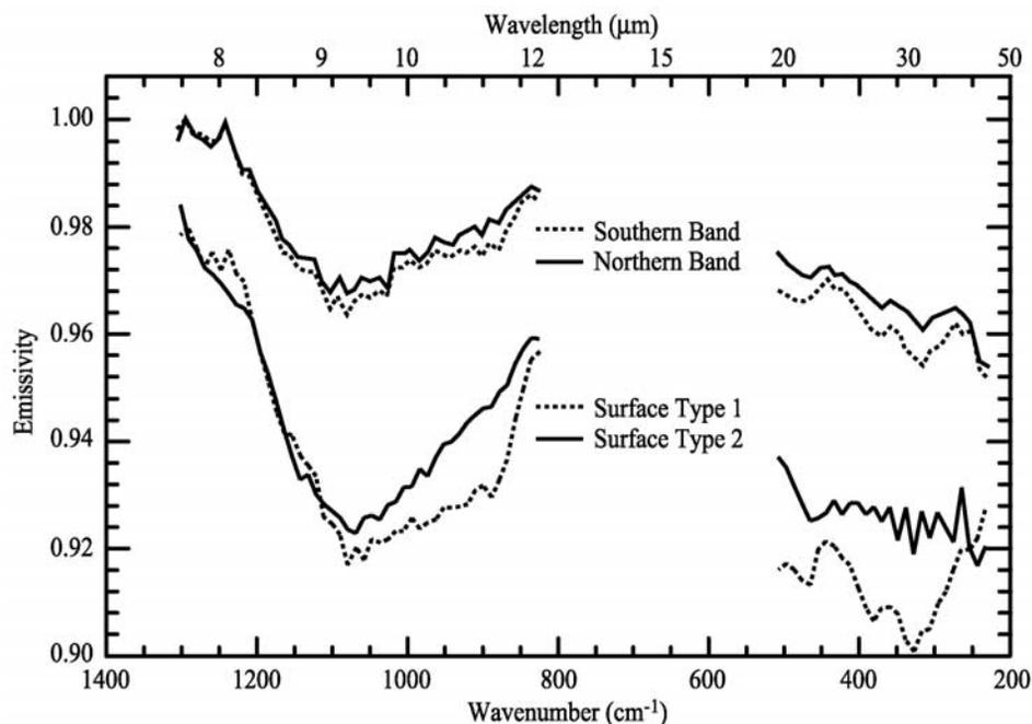
**Figure 4.** Average atmospherically corrected thermal emissivity spectra of the northern and southern transition bands in Acidalia Planitia compared to surface type 1 and type 2 spectral end-members. The southern band is dominated by surface type 1 components ( $\sim 60$  vol %), whereas the northern band is dominated by surface type 2 components ( $\sim 66$  vol %).
