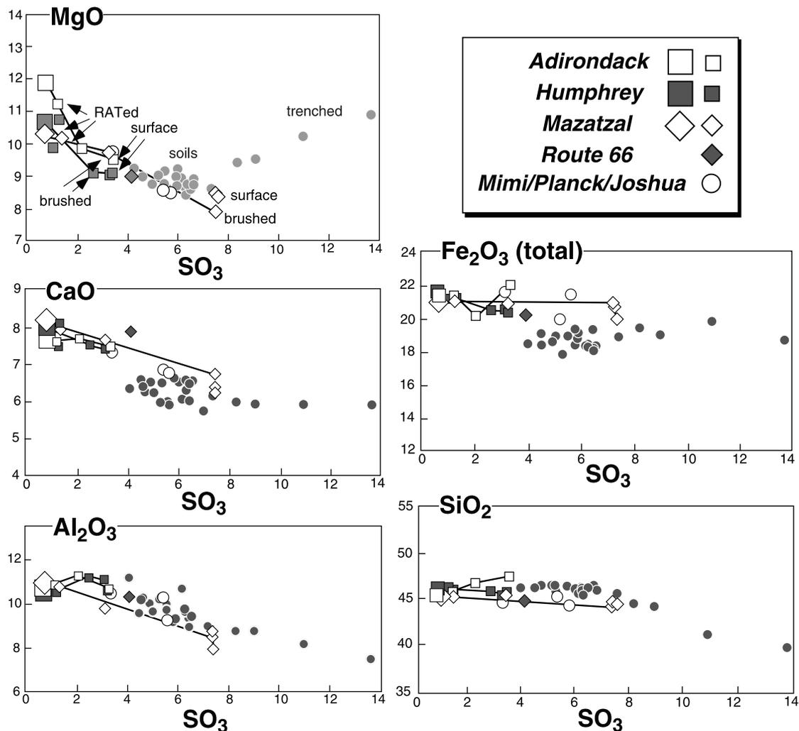
**Figure 8.** APXS analyses of rocks and soils [Gellert *et al.*, 2006], oxides plotted versus  $\text{SO}_3$ . Clean rock compositions (large symbols) are derived by extrapolating from brushed compositions through RATED compositions to 0.3 wt% sulfur (0.75 wt%  $\text{SO}_3$ ). Route 66 (RATED composition) is distinguished from Mimi, Planck, and Joshua (unbrushed compositions).
