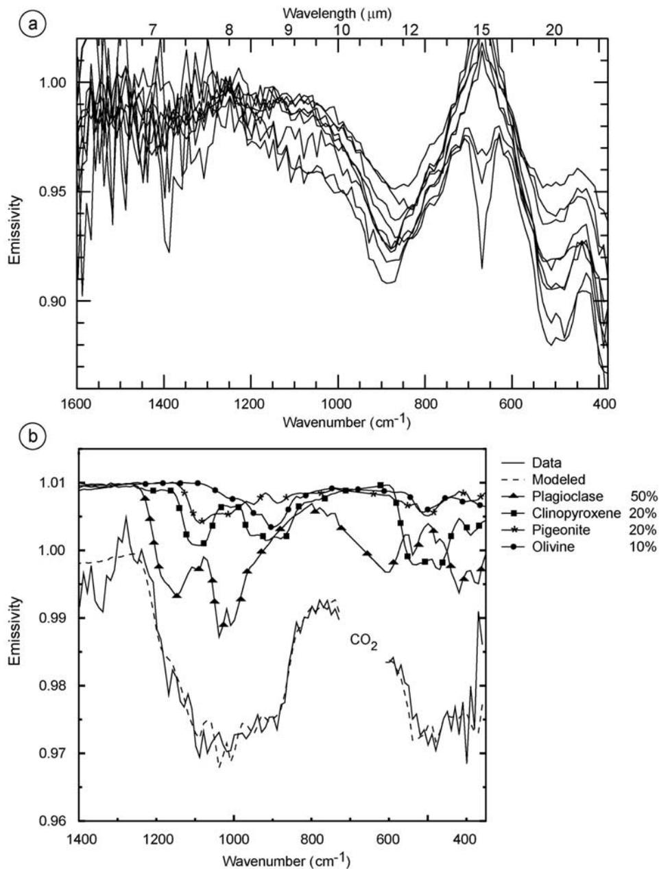
**Figure 7.** MiniTES spectra of Gusev rocks and soils. (a) Spectra of non-dusty rocks are similar, demonstrating that all the rocks on the plains have similar compositions. The absorption band at  $\sim 500 \text{ cm}^{-1}$  results from olivine. (b) Deconvolved spectra of average disturbed soils on the Gusev plains probably reflect the mineralogy of the rocks. CO<sub>2</sub> marks the position of the atmospheric CO<sub>2</sub> band.
