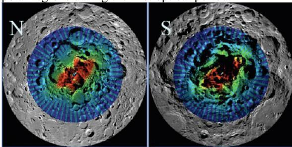
**Figure 2.** Predicted targeted-mode coverage of the polar regions during the first optical period. The colored areas cover the surface poleward of  $80^\circ$ . Blue indicates that the surface will be measured once while red indicates 4 or more measurements.
