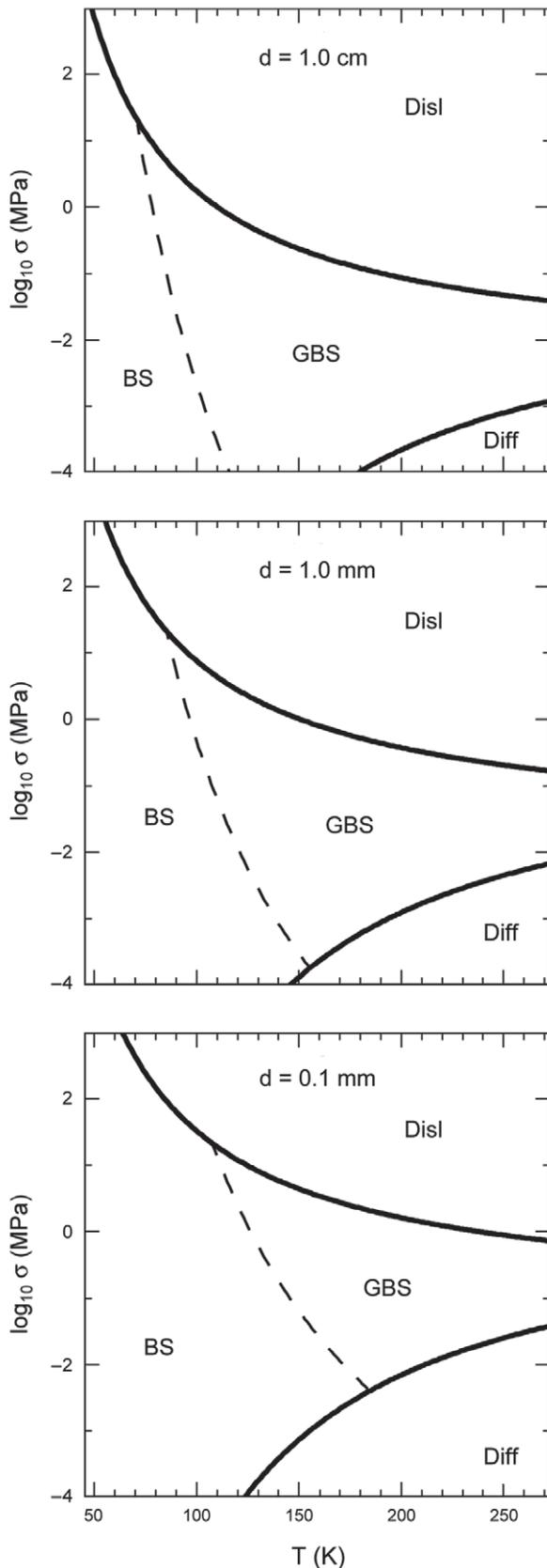
**Fig. 2.** Deformation maps for ice I using the rheology of *Goldsby and Kohlstedt* (2001), for ice with grain sizes of 1.0 cm, 1.0 mm, and 0.1 mm. Lines on the deformation map represent the transition stress between mechanisms as a function of temperature. From *Barr et al.* (2004).
