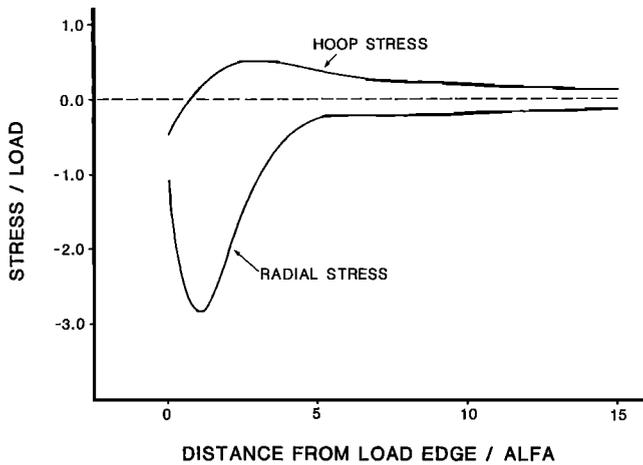
Fig. 15. Radial and hoop stresses as a function of distance from the load edge for uplift in response to an applied negative load. Stress is normalized to the applied load and distance is in units of  $\alpha$ . Negative stress is compressional.
