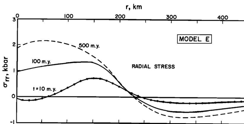
Fig. 18. Surface radial stress  $\sigma_{rr}$  for model E, a combination of uplift heating from model A (Figure 10) and impact heating from model D ( $E_B = 7 \times 10^{32}$  erg and  $s = 50$  km, Figure 16). An elastic blocking temperature  $T_e$  of  $800^\circ\text{C}$  has been assumed.
