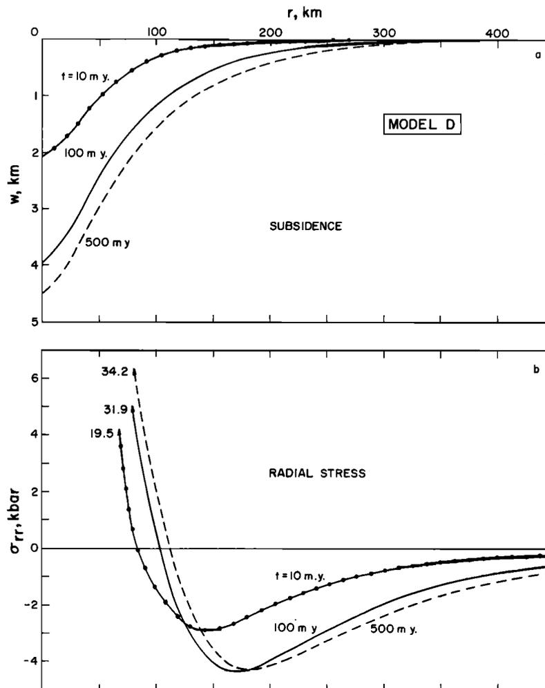
Fig. 17. Surface subsidence  $w$  and radial stress  $\sigma_{rr}$  for model D (Figure 16).
