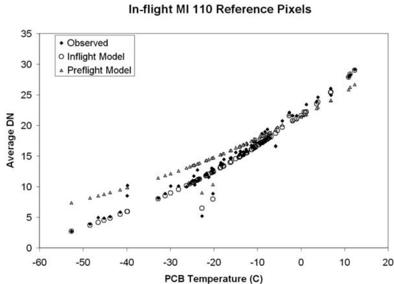
**Figure 4.** Average of observed reference pixel data in samples 4–14 and lines 412–612 compared with models based on preflight and in-flight calibration data. PCB is printed circuit board in the MI electronics box.
