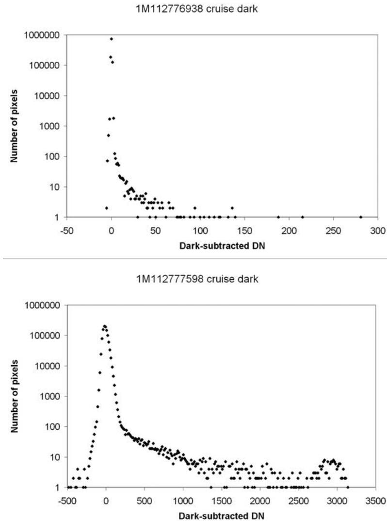
**Figure 3.** Histograms of MI dark current data acquired during first cruise instrument checkout on 30 July 2003. The MI dark current model was used to subtract average dark current variations from each image. (top) Zero-second exposure image. (bottom) One hundred-second exposure image.
