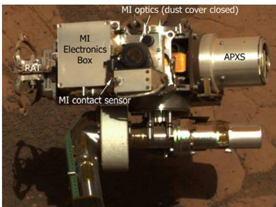
**Figure 1.** Pancam color (filters L4, L5, and L6) image of Opportunity's Instrument Deployment Device (IDD) turret (about 30 cm across), taken on sol 405 with illumination from top. Bright vertical lines are artifacts caused by blooming of saturated pixels.
