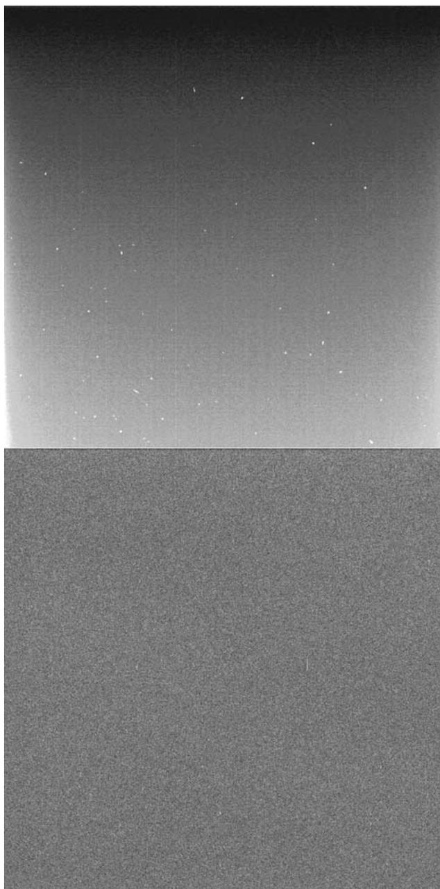
**Figure 2.** Microscopic Imager (MI) dark current images taken during first cruise instrument checkout on 30 July 2003. Contrast is enhanced to emphasize subtle features. (top) Zero-second exposure image 1M112776938 showing temporary radiation effects. (bottom) One hundred-second exposure image 1M112777598.
