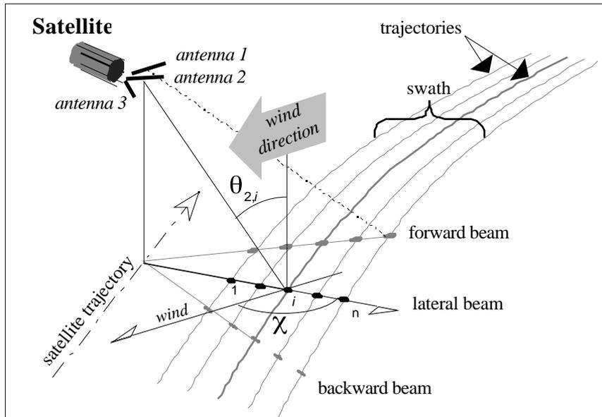
**Figure 2 :** Definition of the geometry of the scatterometer observations.
