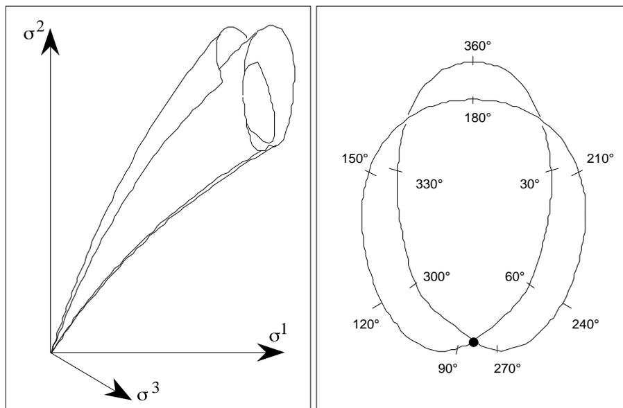
**Figure 3 :** (a) Functional for computing the wind speed and direction as a function of the  $\sigma^0$  measured by the antennas (b) Graph obtained for a section at constant wind speed.
