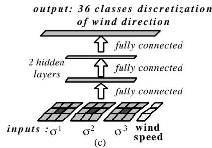
**Figure 10** : network representing the output direction using the classifier mode; the output range is discretized in 36 classes, each one representing  $10^\circ$ .
