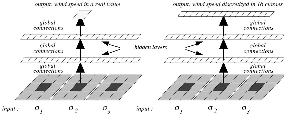
**Figure. 9 :** two different networks representing the wind speed respectively using the real (left) and the classifier (right) modes .
