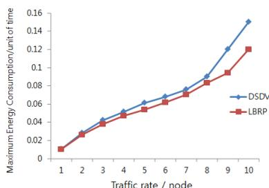
Fig. 2. Comparison of the energy consumption between LBRP and DSDV
