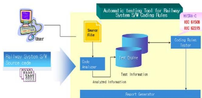
Fig. 1. Outline of the automated testing tool for software coding standard
