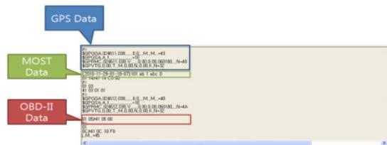
Fig. 2. GPS, MOST, and OBD-II data outputted
