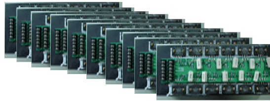
Fig. 3. The developed linear power amplifier PCB(500W*10=5kW)
