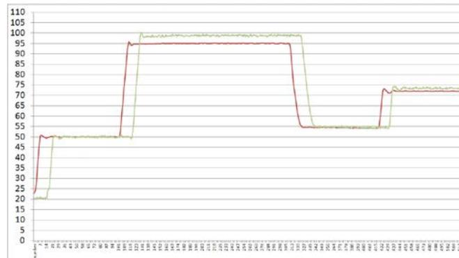
**Fig. 3.** Measured temperature of micro PCR chamber.
