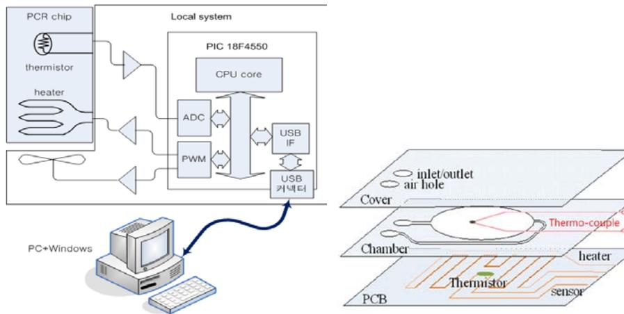
Fig. 1. PCR Chip drive system
