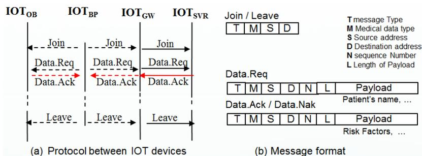
Fig. 3. Collaboration model between PHDs for the smart healthcare service
