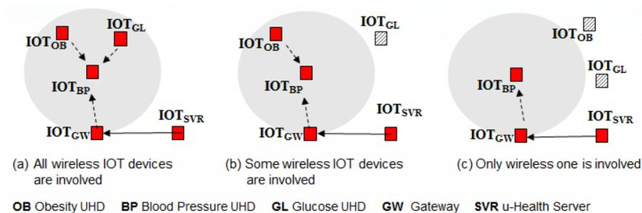
Fig. 2. Collaboration model between IOTs for the smart healthcare service
