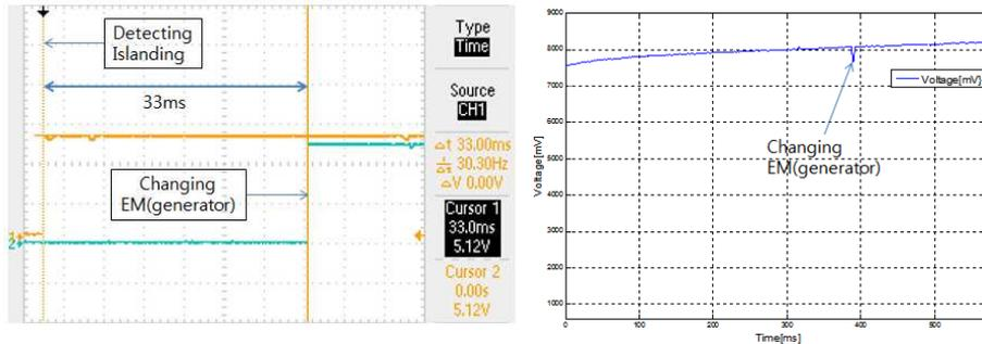
Fig. 4. The Detecting time of islanding and EV charging voltage at occurred islanding
