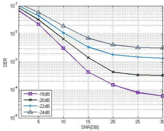
Fig. 3. BER Performance of watermarking signal among received signal
