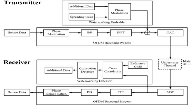
Fig. 1. Block diagram of OFDM communication system and additional data transmission scheme in the underwater channel
