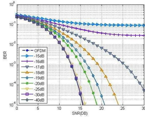
Fig. 2. . BER Performance of OFDM signal among received signal
