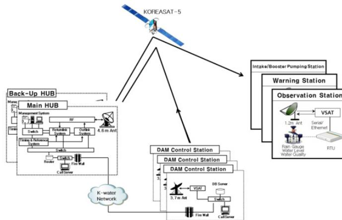
Fig. 1. Diagram of K-water's Satellite Communications Network
